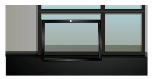
Place the assembled IndowPRO frame into the window frame.
